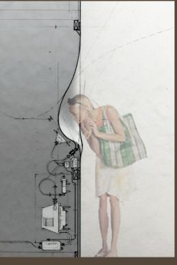
DSR made a careful study of mechanisms for the delivery of the fragrances. They used a pump system manufactured by German company Scent Communication, in which an essential oil saturates beads packed into cartridges and a pump distils the fragrance by forcing air over the scented polycarbonate beads.
