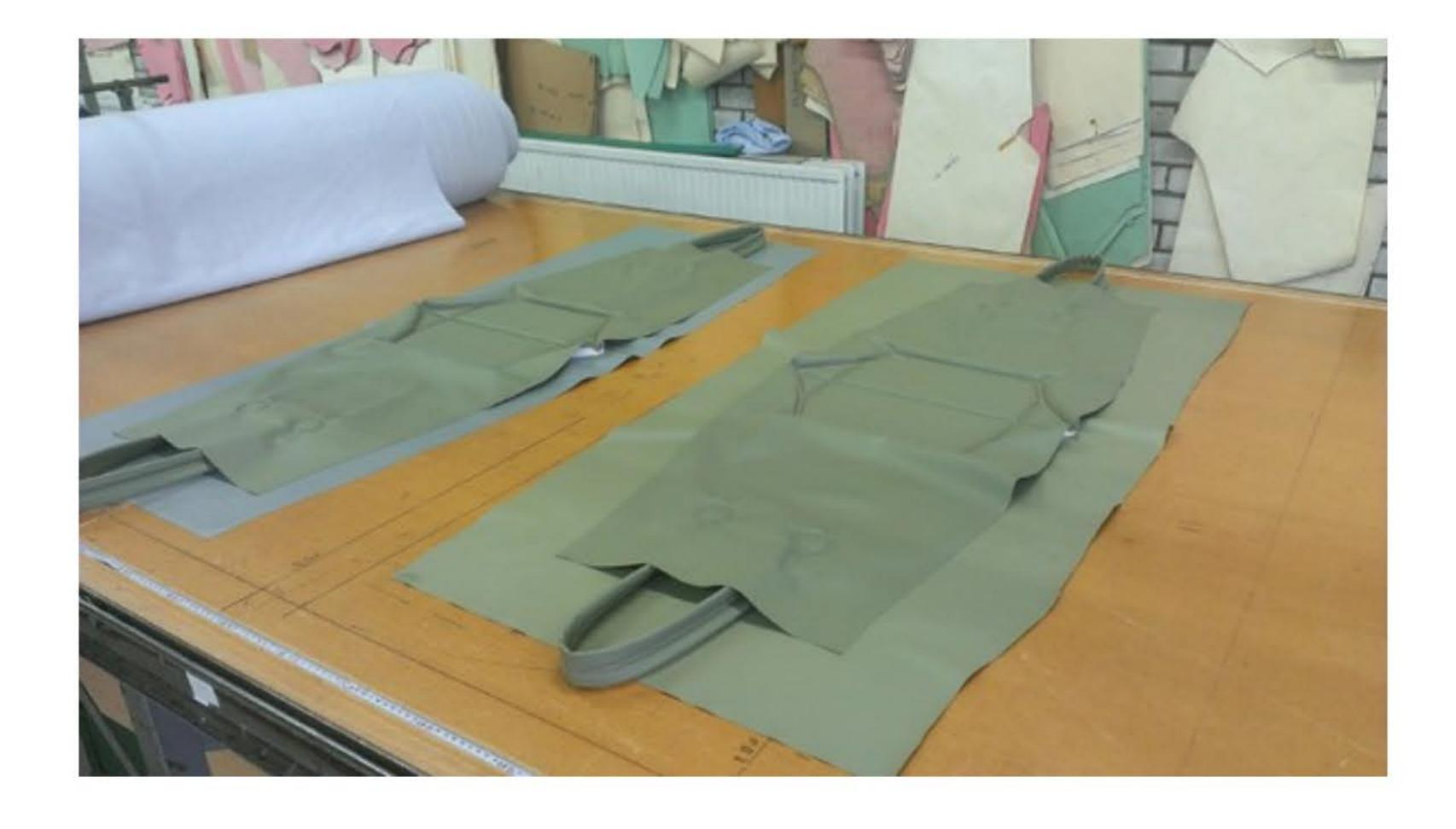
The panels were "sewn" together using a microwave-like, high-frequency welding technique. With Crease-made from garden chair PVC wire-de Groot determined the bag's volume by strategically welding folds into its bottom and sides, an innovation that makes the bag both unusual and good-looking.
